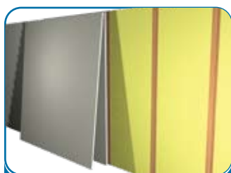
Remove the inner panel(s) and replace insulation as required.
